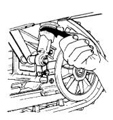
To adjust, use the adjustment key supplied and turn the spring collar accordingly.
