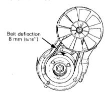
If belt seems damaged or if tension is incorrect, contact your dealer immediately.
