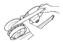
Slip the belt out from the drive pulley and remove completely from the vehicle. To install the drive belt, reverse the procedure.
