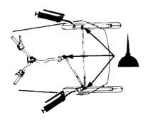
Oil spring coupler bolts, ball joints and steering column bushings.
