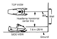
With the suspension correctly adjusted, the rider seated on the vehicle and the high beam ON check that the center of high intensity zone of high beam is 50 mm (2") below horizontal line of headlamp height.
