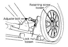
NOTE: Track tension and alignment are inter-related. Do not adjust one without the other.
