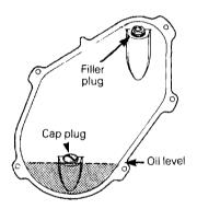
The oil should be level with the bottom of the oil level orifice.
