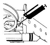
CAUTION: When lubricating the drive axle bearing, do not apply excessive grease as the seal will be pushed out of its housing. Check seal position with finger.
