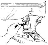
To adjust, use the adjustment key supplied and turn the spring collar accordingly.
